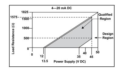
Figure 2-3. Supply Voltage vs. Load.
